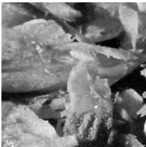
Fig. 9 – Detaliu amestec talaj apa de sticla in care se observa granulele de silicat
